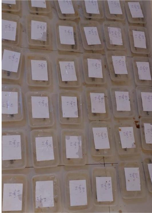
**Fig. 3. Vessels used to assess the loss of mass of steels after immersion in a corrosive solution**
