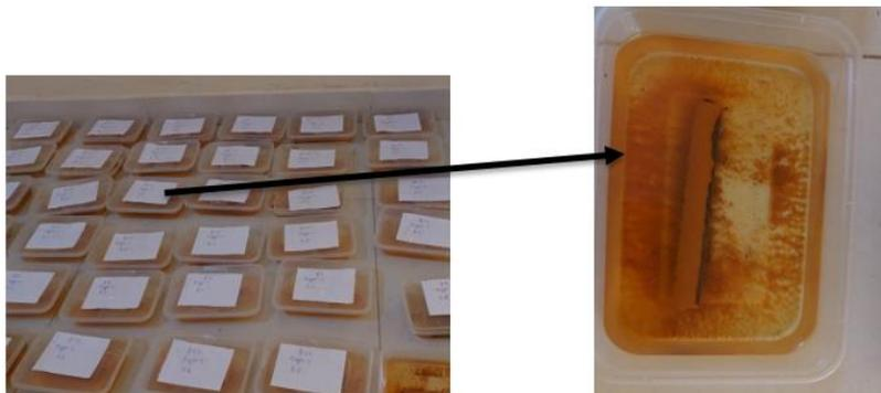
Fig. 4. Colour change of corrosive solution at measurement time
