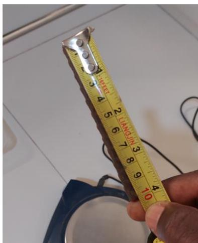
**Fig. 2. Measurement of sample length for mass determination**
