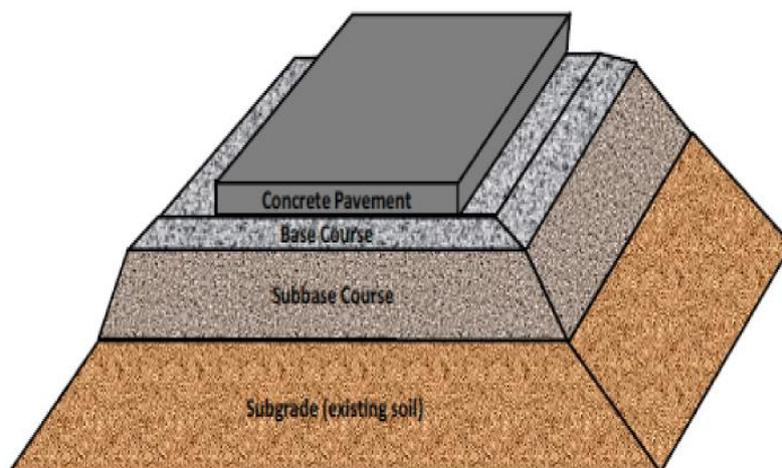
*Fig. 5. Typical cross-section of a pavement structure and terminology of the different layers*
