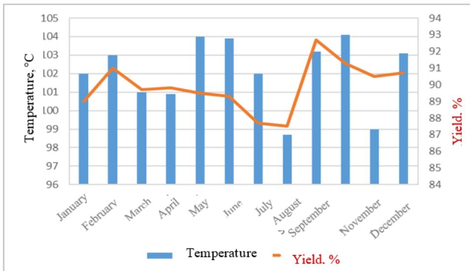
Fig. 8. Changes in alumina yield as a function of etching temperature
