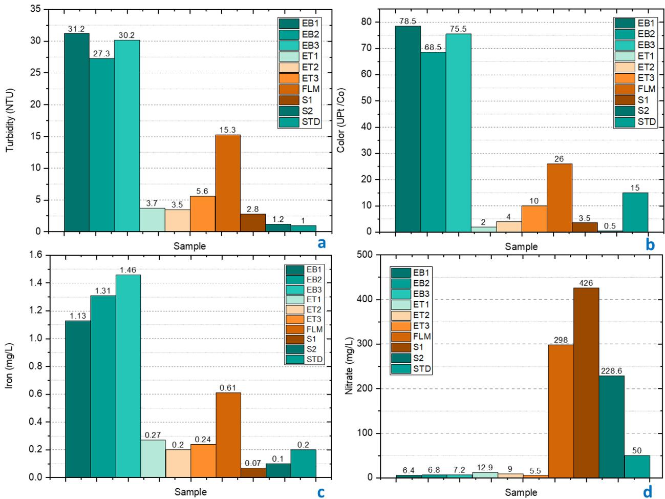
**Fig. 2.** Variation of element values in the analyzed samples. (a) Turbidity, (b) Color, (c) Iron and (d) Nitrate. STD symbolizes the value guiding the WHO and the European Union
