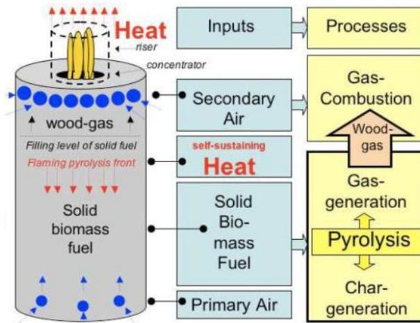
Fig. 2. Basic design of Top-Lit Updraft gasifier stove [18]
