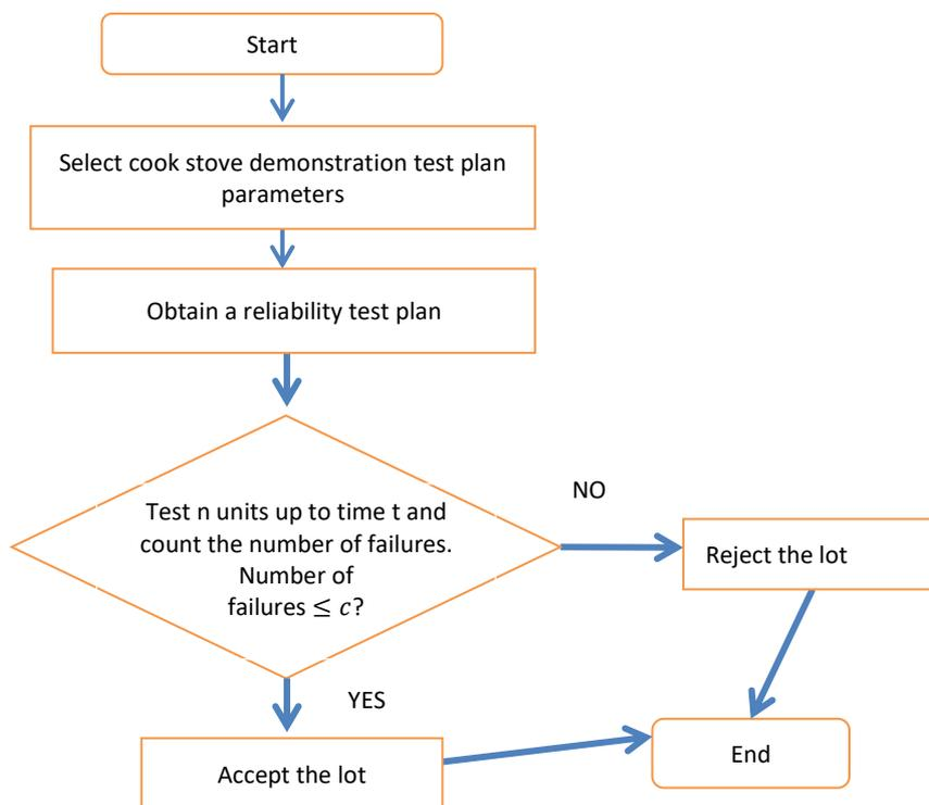
Fig. 4. Flowchart of reliability demonstration test plan
