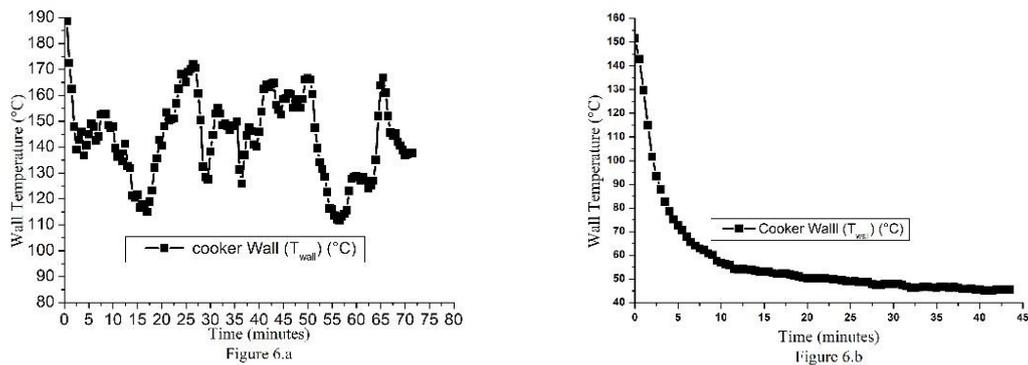
Fig. 6. Temperature evolution of the vertical wall of the cooker before and after heating
