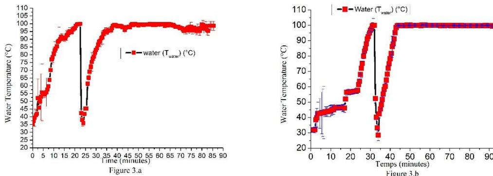
Fig. 3. Boiling temperature of water with lid (left) and without lid (right)
