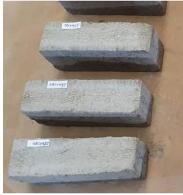
**Fig. 13. Blocks after abrasion test**
