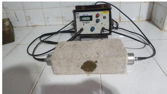
**Fig. 6. Ultrasonic pulse velocity tester**
