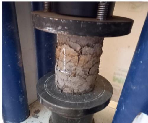
**Fig. 5. Simple compression test device**
