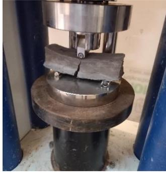
Fig. 6. Testing device for 3-point bending
