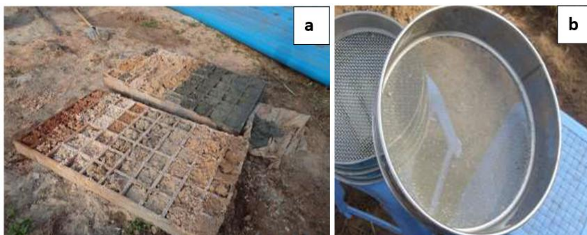
Fig. 3. Equipment used for particle size measurements: a) boxes containing soil samples taken during drilling; b) sieves used for particle size analysis
