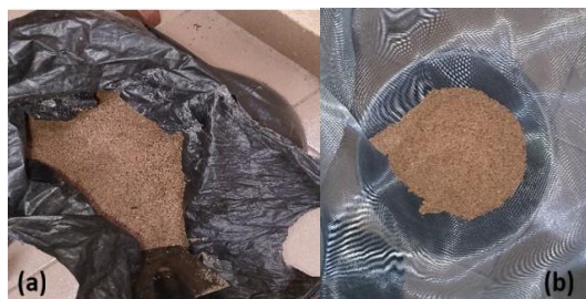
Fig. 2. Sanaga Sand (a) Raw sand (b) Sieved sand ( d < 1\text{mm} )
