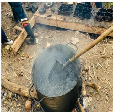
**Fig. 9. Melted plastic waste mixed with sand**
