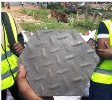
**Fig. 3. A model of eco-friendly paving block made from plastic waste**
