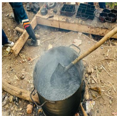
Fig. 9. Melted plastic waste mixed with sand
