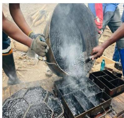
**Fig. 11. Exposure to fumes during the molding of melted plastic**
