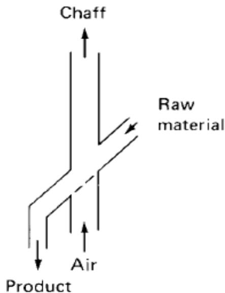
**Fig. 1.1.2 Separation of chaff from grain by aspiration cleaning**
