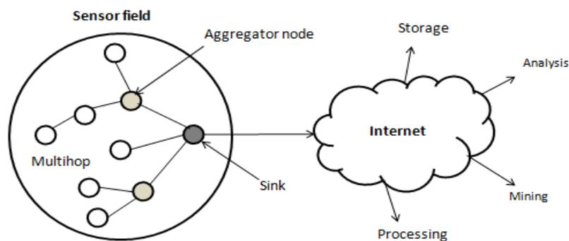
Fig.1. Architecture of Wireless Sensor Network
