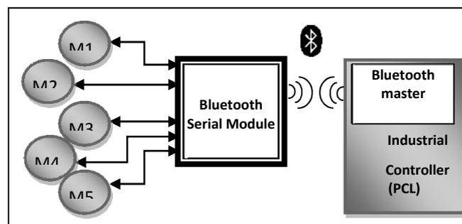
**Fig. 8. Bluetooth communication between a device and a system of supervision**
