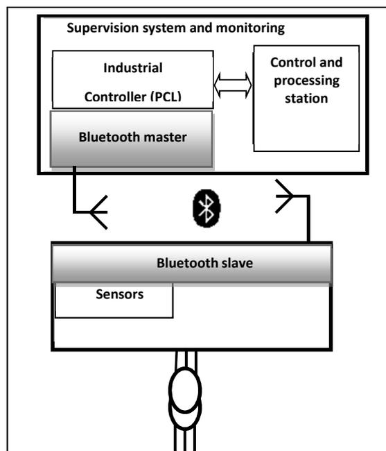
Fig. 6. Synoptic of an industrial chain with Bluetooth transmission
