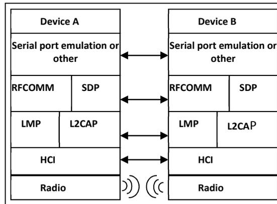
Fig. 5. Serial Port Profile model
