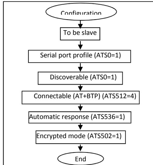
**Fig. 10.** Organization chart for the configuration of Bluetooth module.
