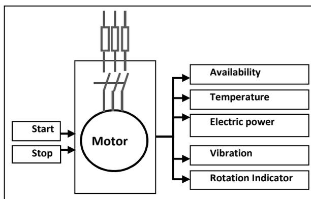
Fig. 2. Signals associated to a motor
