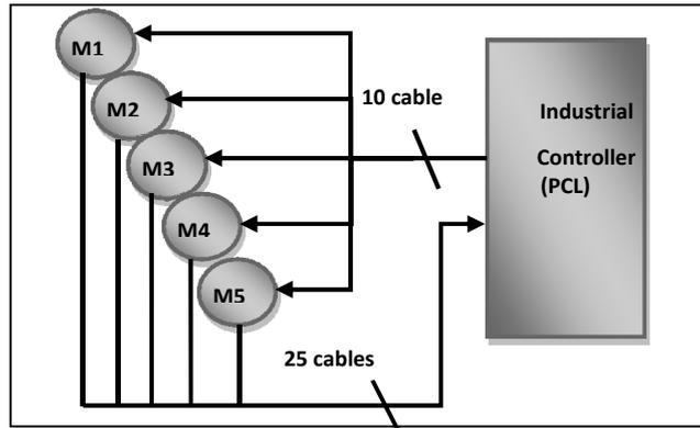
Fig. 3. Cabling of an industrial machine (5 motors)
