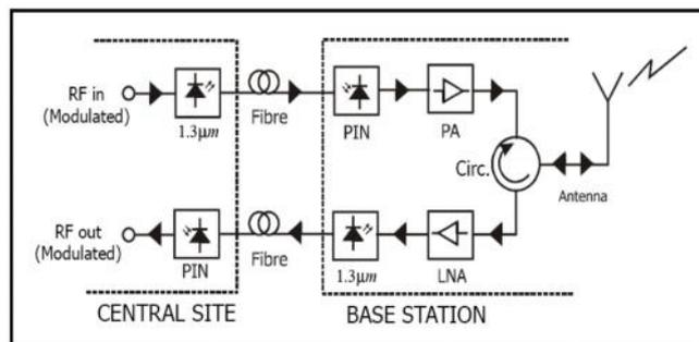
*Fig.1 Radio over Fiber System*
