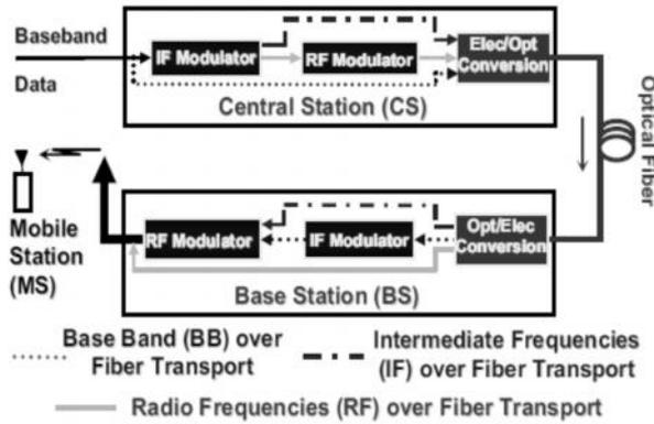
Fig 2 Transport schemes for Fiber/Wireless systems
