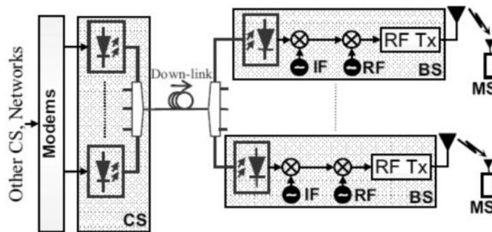
Fig.3 IF to RF up-conversion at the base stations
