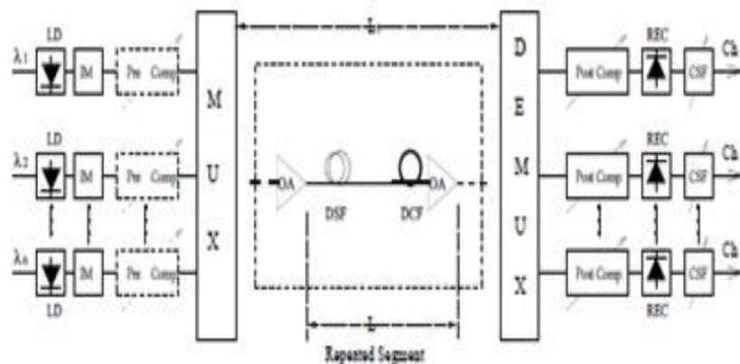
Fig 4 configuration of typical WDM transmission system including the wave
