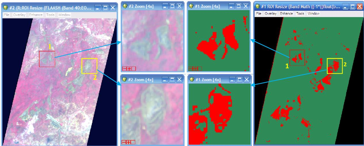
**Fig. 4.** *Fig 4: Showing the final result of Iron ore mines of Noamundi areas. Hyperion Image (Left) and comparative mine areas (Right)*
