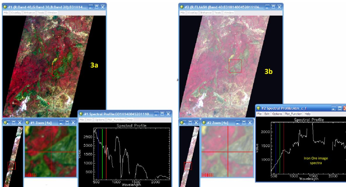
Fig. 3. Showing the spectral profile of Iron ore mining areas of before and after atmospheric correction. 3a: Before atmospheric Correction and 3b: after atmospheric Correction
