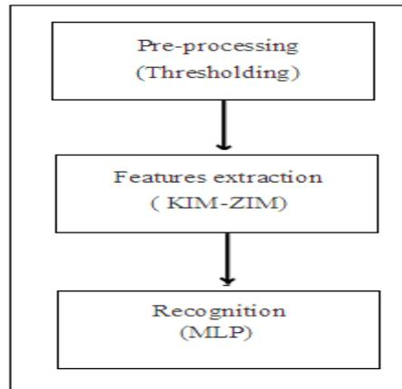
Fig. 1: System for Arabic characters recognition.
