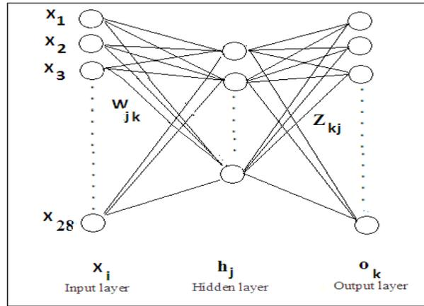
Fig. 2: The multi-layer perceptron (MLP).
