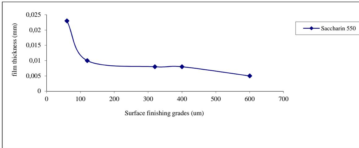
Figure 4: Effect of SFG on film thickness on NST50-2 steels (with 0.5g/l saccharin)
