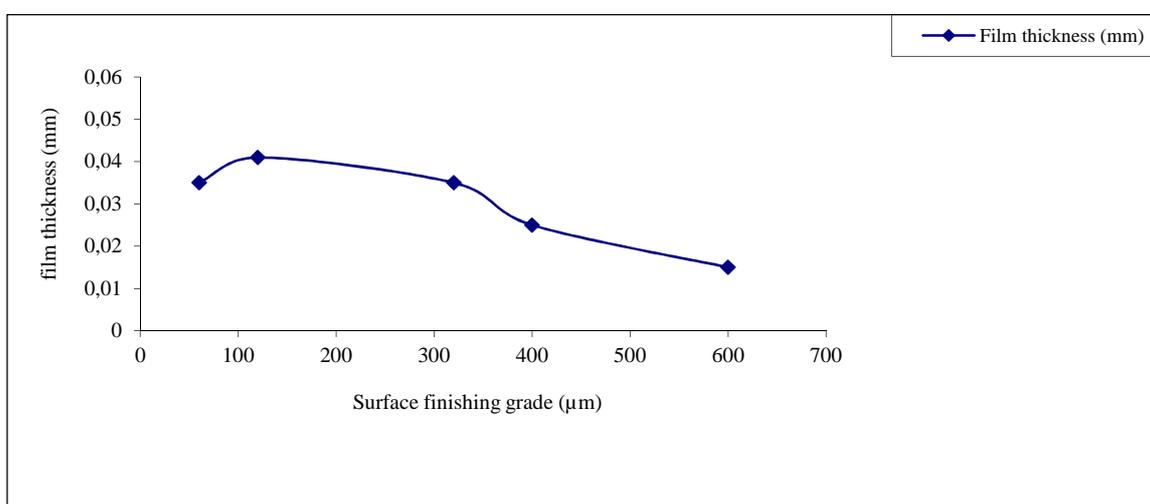
Figure 2: Effect of SFG on copper film thickness (in bath without additive)
