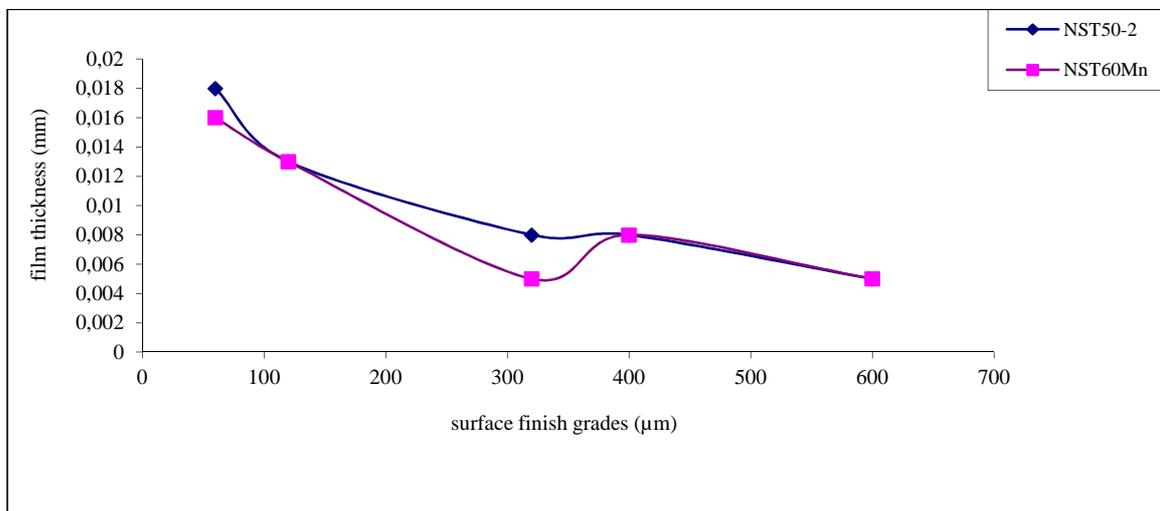
Figure 5: Effect of SFG on film thickness on NST50-2 and NST60Mn (with 0.5g/l saccharin)
