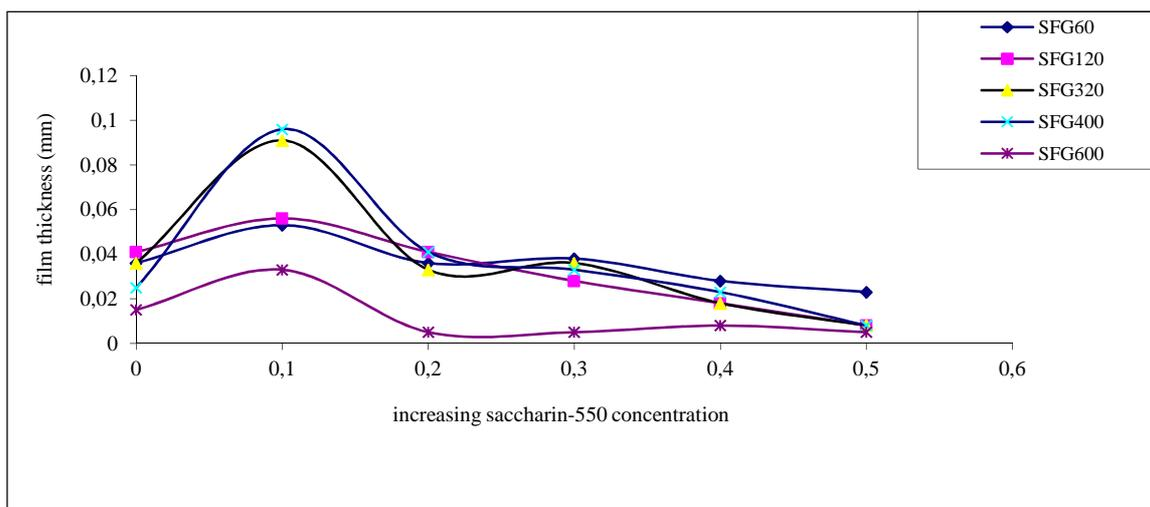
Figure 3: Effect of varying SFG and saccharin concentration on film thickness on NST50-2
