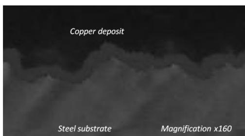
**Plate 4: Optical microscopic view of copper film on 600 $\mu\text{m}$  polished substrate.**
