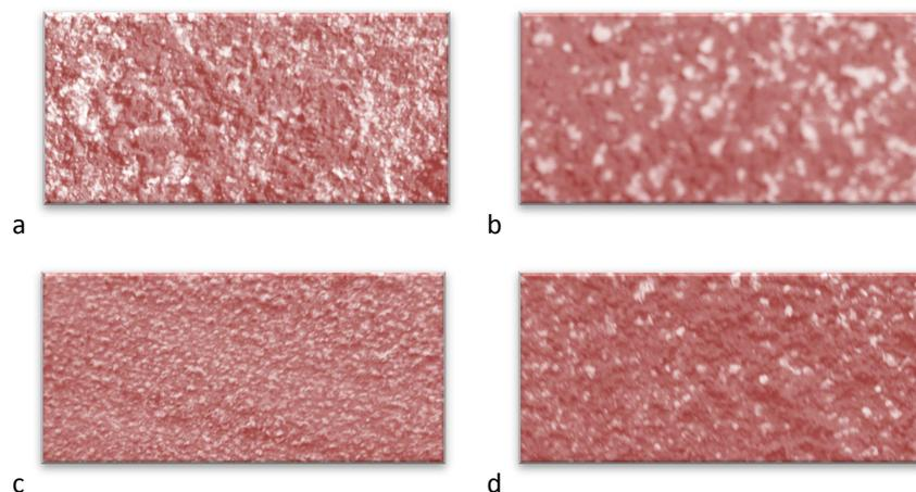
**Plate 5: Optical macrographs of copper film on (a) 60µm, (b) 120µm, (c) 320µm and (d) 600µm polished steel substrates.**
