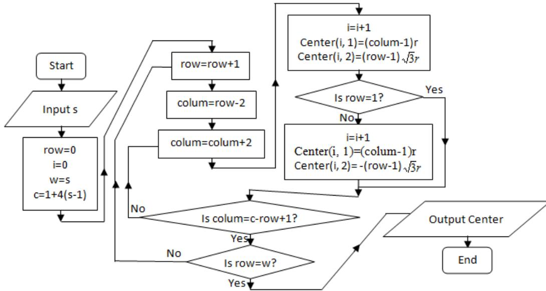
Fig. 6. Flowchart for the Arithmetic and Logical Model of Hexagonal Shaped Stranded Conductor
