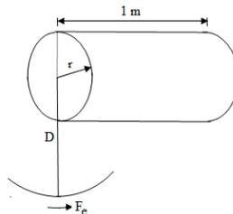
Fig. 2. A Cylindrical Conductor External Flux
