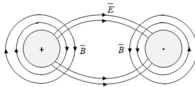
Fig. 1. Magnetic and Electric Fields Associated with Conductors
