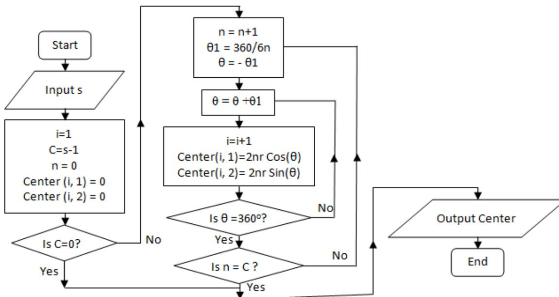
Fig. 8. Flowchart for the Arithmetic and Logical Model of Circular Shaped Stranded Conductor
