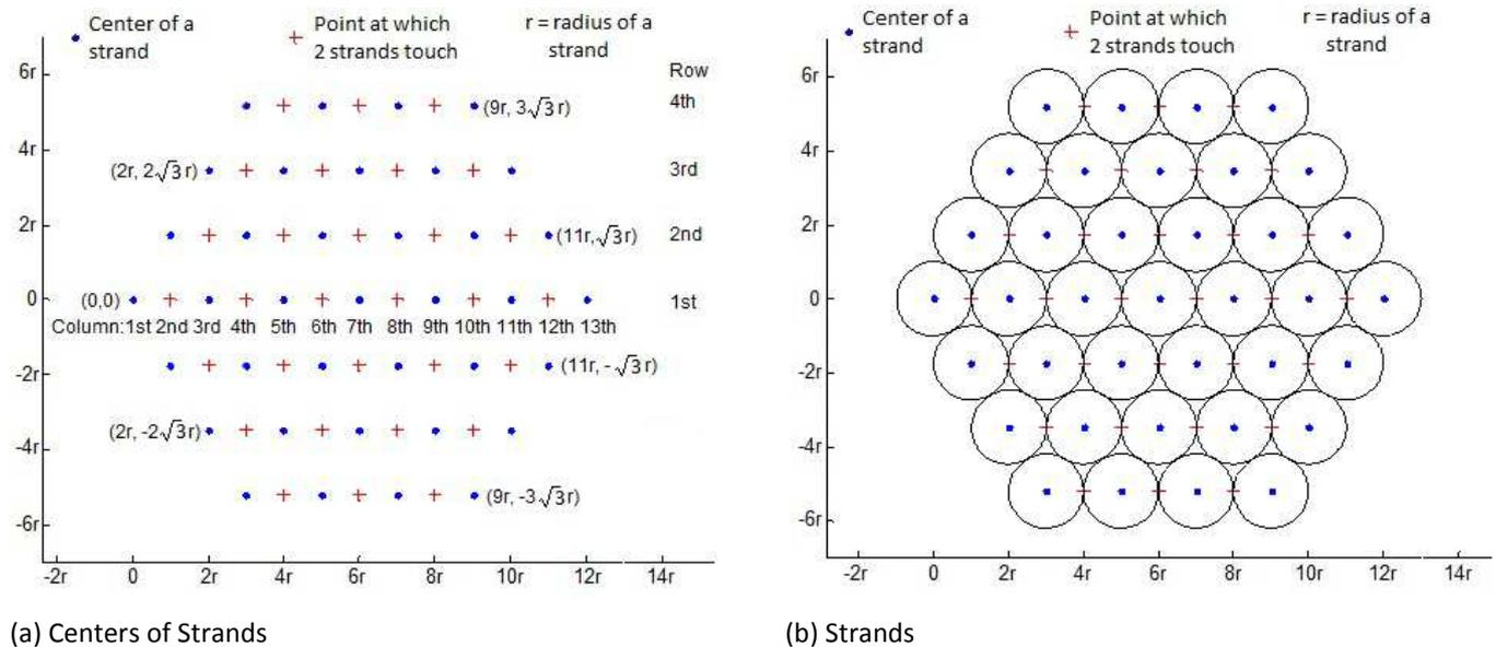
Fig. 5. Hexagonal Shaped Stranded Conductor with  $s = 4$ ,  $N = 37$ ,  $w = 4$  and  $c = 13$
