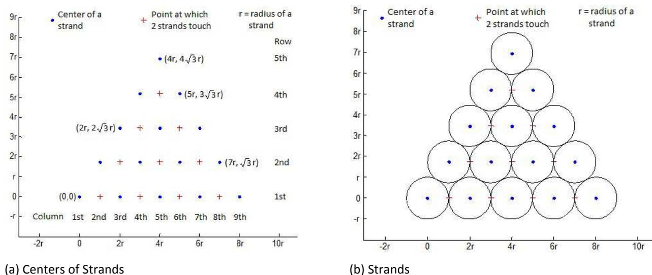
Fig. 3. Triangular Shaped Stranded Conductor with  $s = 5$ ,  $N = 15$ ,  $w = 5$  and  $c = 9$
