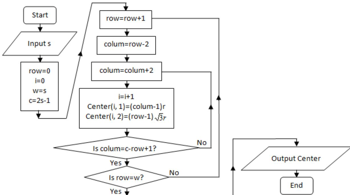
Fig. 4. Flowchart for the Arithmetic and Logical Model of Triangular Shaped Stranded Conductor
