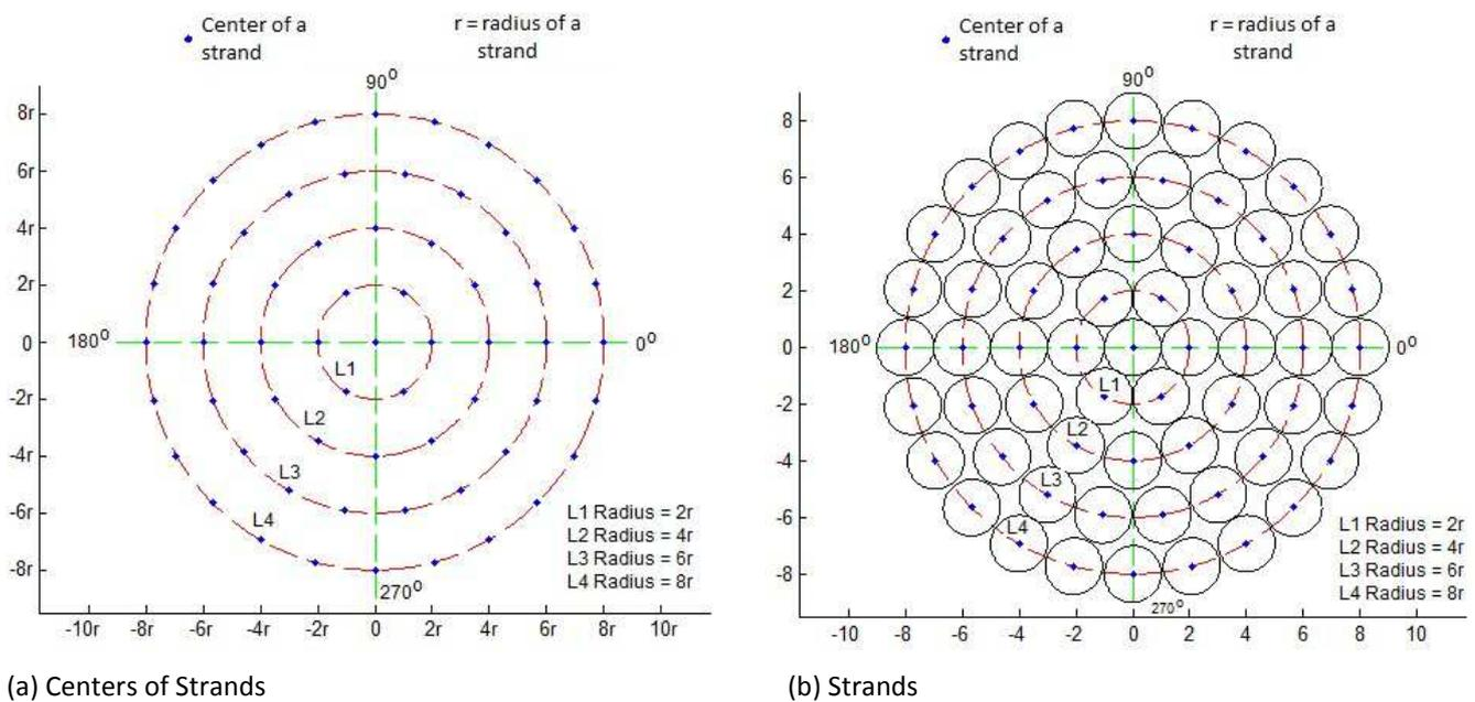
Fig. 7. Circular Shaped Stranded Conductor with s = 5, N = 61 and C = 4
