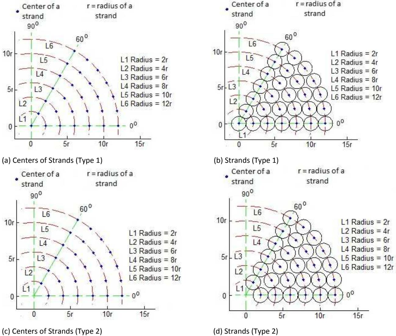
Fig. 9. Circular Shaped Stranded Conductor with  $s = 5$ ,  $N = 61$  and  $C = 4$
