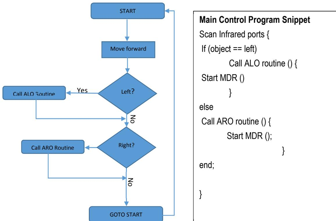
Fig 2.0 (a) Flow chart diagram of Robot Search routine (b) Control code snippet
