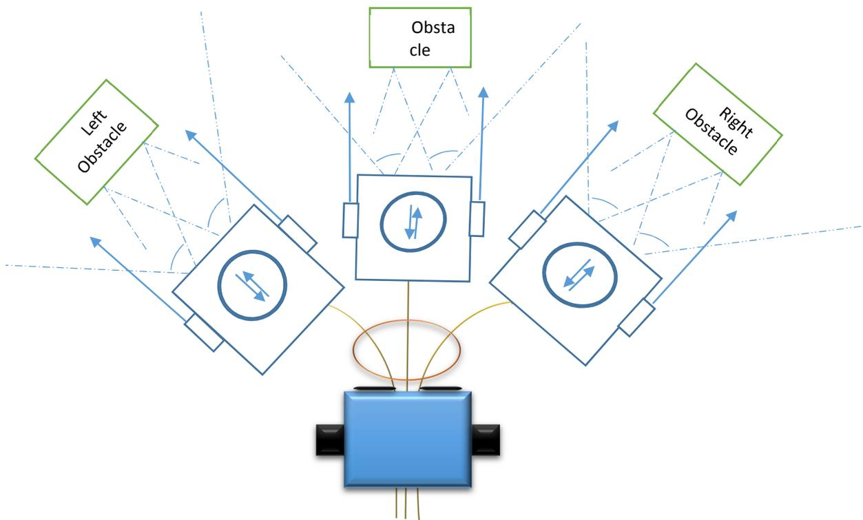
Fig 3.0 Robot Multi directional Search path
