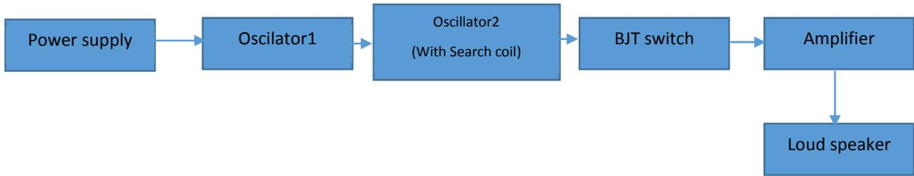
Fig 5.0 Metal detector block diagram [4]
