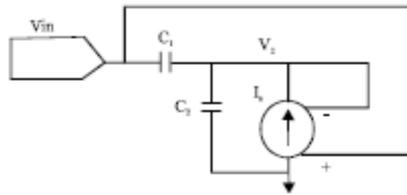
Fig 6.0 Colpitts Oscillator Model [3]
