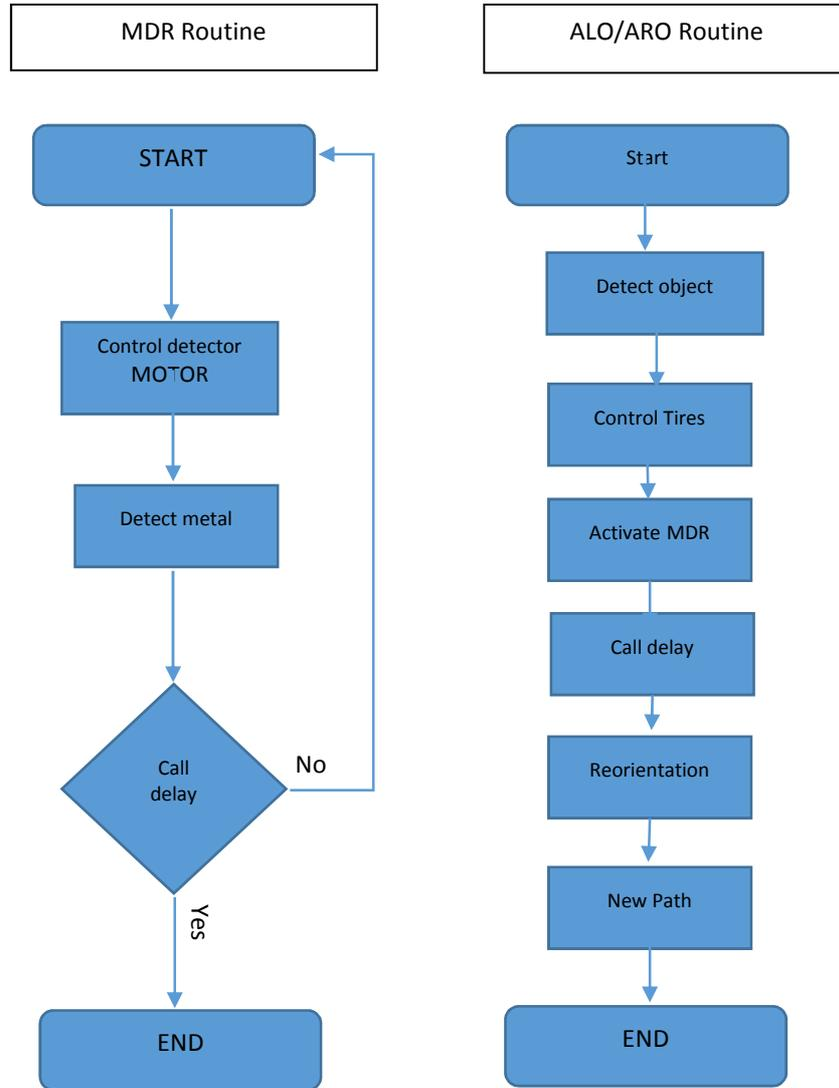
Fig 4.0 (a) Metal Detection routine (b) Obstacle Avoidance and Coil search routine
