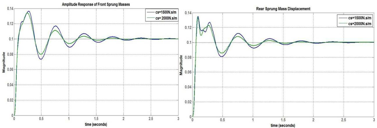
Fig. 7 Amplitude Response of Half Car Model Front Sprung Mass Fig.8. Amplitude Response of Half Car Model Rear Sprung Mass
