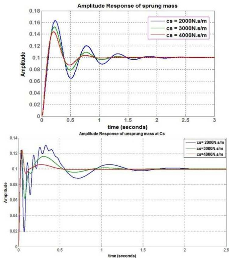
Fig. 3 Amplitude Response of Quarter Car Model Sprung Mass Fig. 4 Amplitude Response of Quarter Car Model UnSprung Mass
