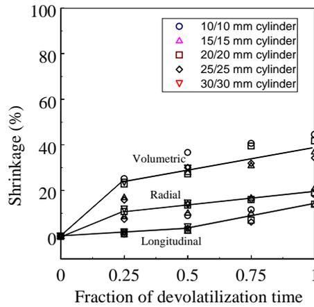
Fig.5. Progress of shrinkage during devolatilization.  $T_{bed} = 750\text{ }^{\circ}\text{C}$ .
