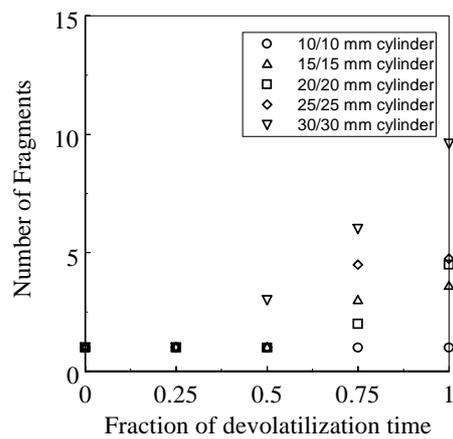
Fig.6. Timing of fragmentation at a bed temperature of  $950\text{ }^{\circ}\text{C}$ .
