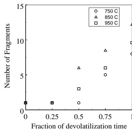
Fig.7. Timing of fragmentation of a  $30/30\text{ mm}$  cylinder at different bed temperatures
