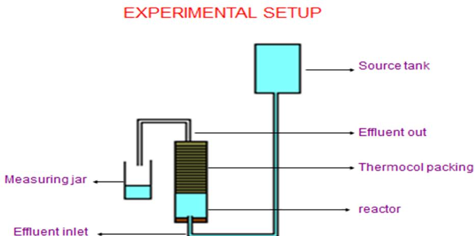
Fig. 1. Experimental Setup Of HUASB Reactor Design
