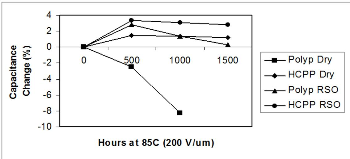
Fig. 1. Performance of Five Micron Segmented Film In Capacitors
