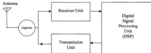
Figure 2.1: Block Diagram of UWB Transceiver
