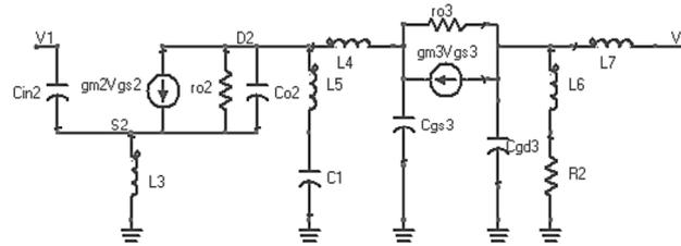
Figure 4.4: Equivalent Circuit for Cascade Stage
