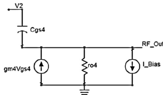
Figure 4.5: Equivalent Circuit for Output Stage
