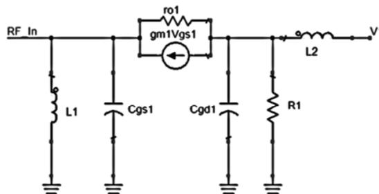
Figure 4.3: Equivalent Circuit for Input Stage
