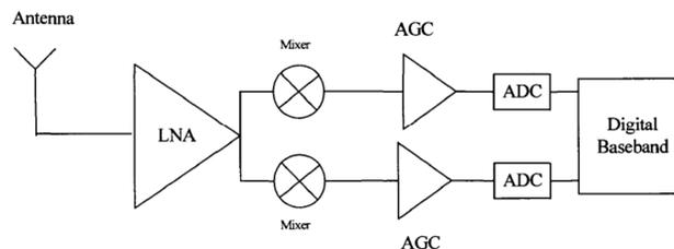
Figure 2.2: Block diagram of receiver
