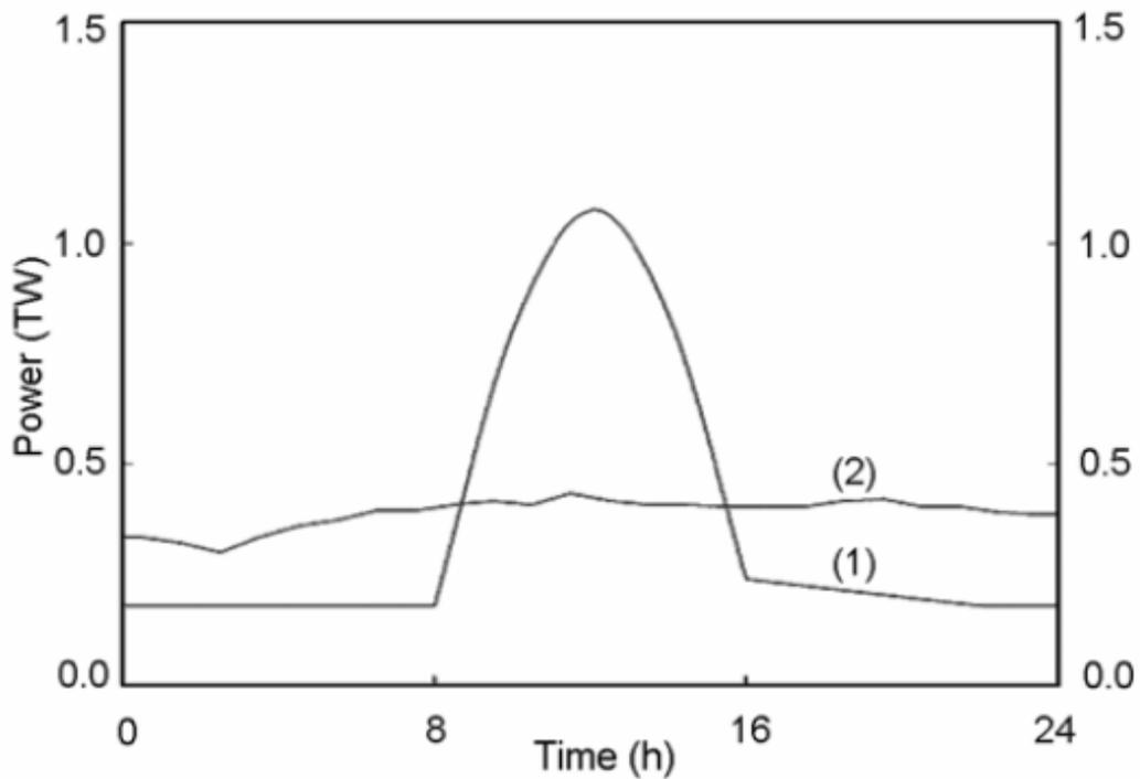
Fig. 2. Comparison of diurnal variation of production (curve 1) and demand (curve 2) over a typical sunny day.
