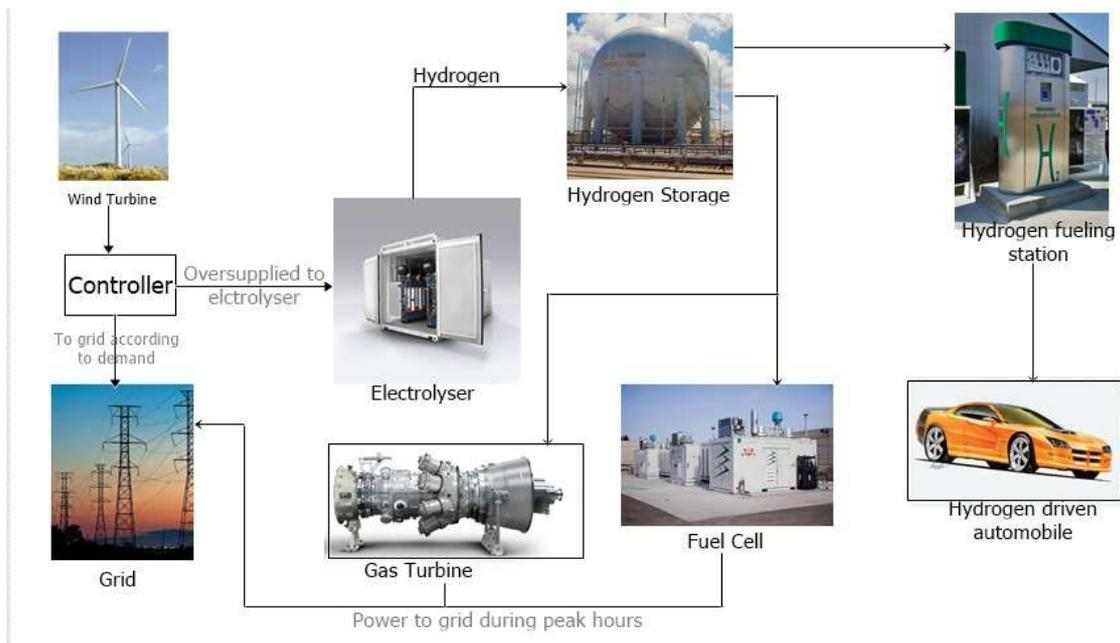
**Fig. 5. A flow chart of Hydrogen production from wind and its utilization**
