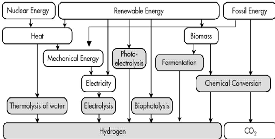
Fig. 1. Hydrogen production methods
