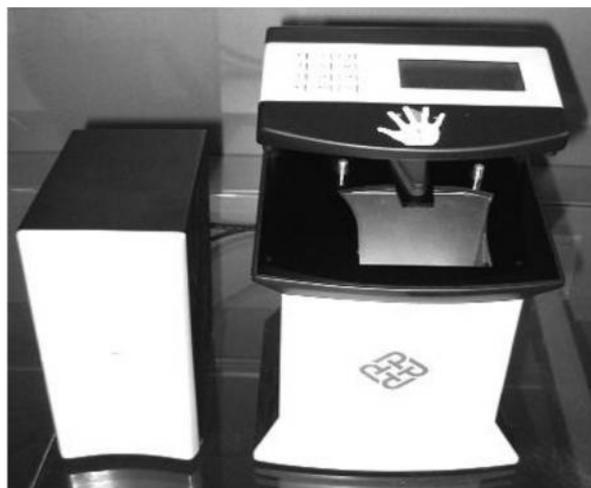
*Fig. 2. CCD based palm print scanner*
