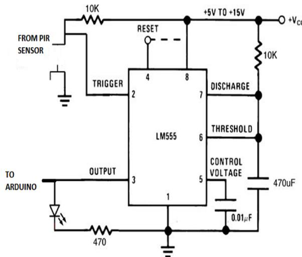
Fig. 2. Circuit Design for an LM555 monostable mode
