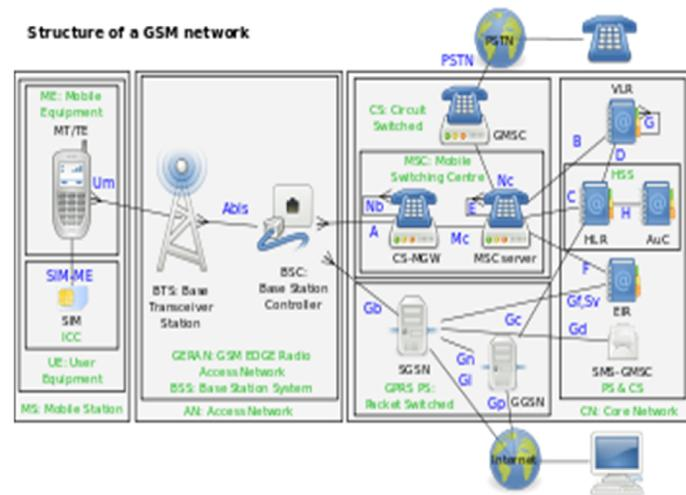
Fig. 3b. GSM network structure
