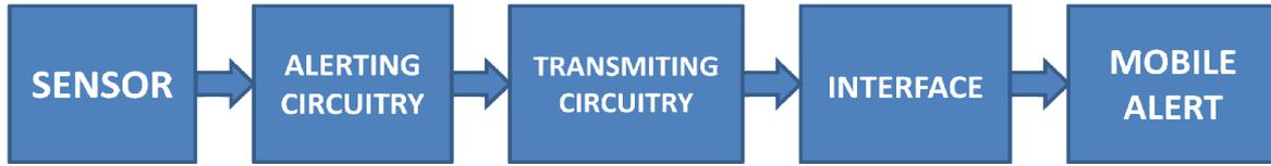
Fig. 1. Block diagram of the burglar alarm system
