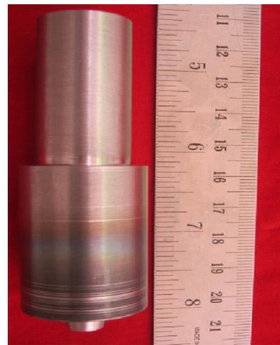
Fig.1d: Tungsten based alloy tool
