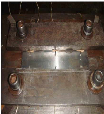
Fig.1e: Thermocouple location
