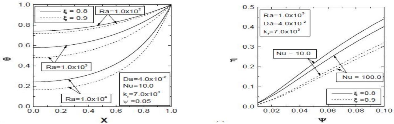
Fig.4.1.2 Variation of temperature excess to distance and efficiency to length to radius ratio
