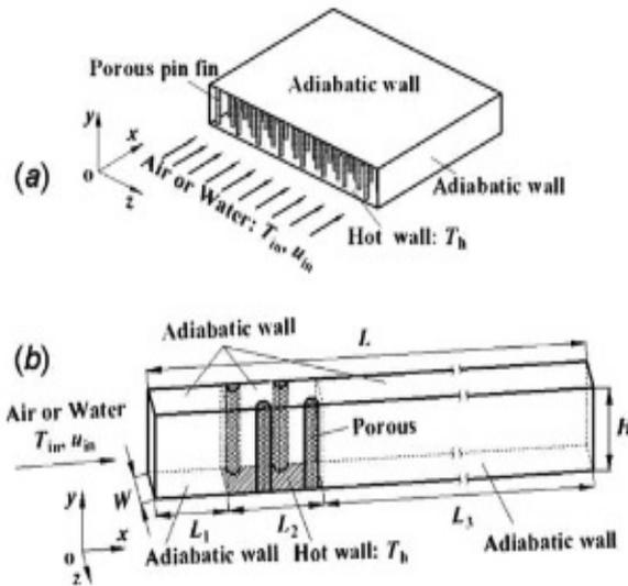
Fig 3.1.1 Porous pin fins as heat exchangers
