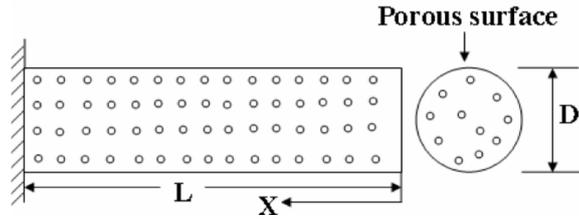
Figure 3: shows a porous fin of length L having pores in it.
