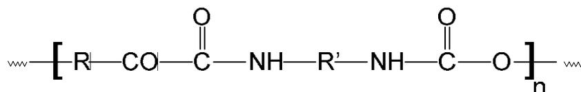
Fig.2. Polyurethane formed from di hydroxyl compound [1]
