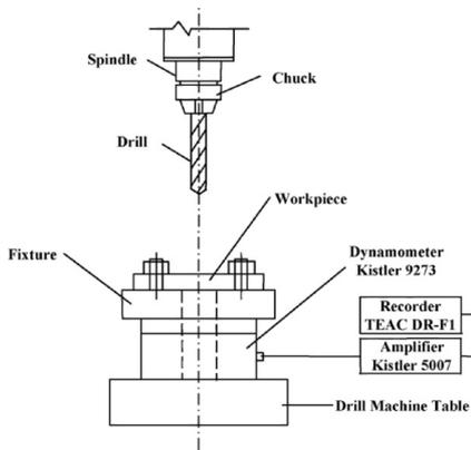
Fig. 3 – Schematic of drilling set-up [6]
