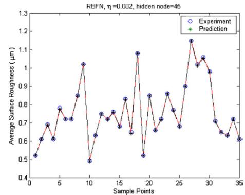
Fig. 5 – Comparison of surface roughness between prediction and experiment. [6]
