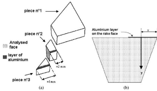
**Fig. 6. Section of the carbide tool insert analysed. [30]**
