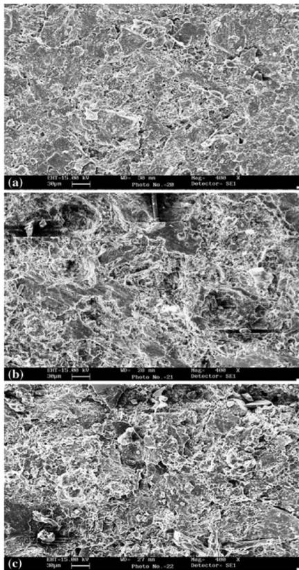
Fig. 9 SEM photographs of workpiece materials before drilling a 50% Alumina, b 60% Alumina and c 70% Alumina [23]
