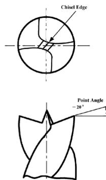
Fig. 4 – Geometry of candle stick drill [6]
