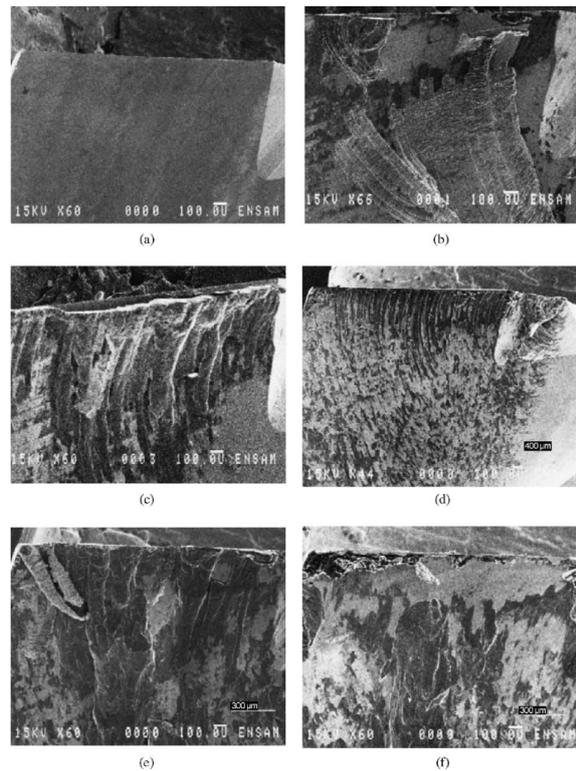
**Fig. 8. SEM observations of the aluminium adhesion on the surface of the optimised carbide drill. The cutting conditions are:  $V = 60 \text{ m/min}$ ;  $f = 0.16 \text{ m/min}$ ; (a) new drill, (b) after 1 hole, (c) after 10 holes, (d) after 48 holes, (e) after 96 holes, (f) after 200 holes. [30]**
