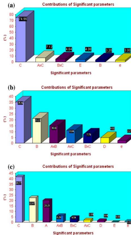
Fig. 10 Bar graphs. A Workpiece, B tool, C grit size, D power rating, E slurry concentration. [23]
