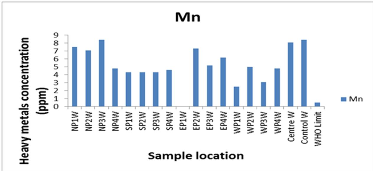
Fig 3.10 A plot of manganese concentration against sample location during wet season
