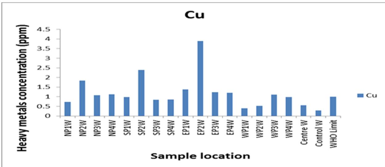
Fig 3.08 A plot of copper concentration against sample location during wet season
