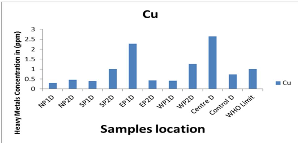
Fig 3.05 A plot of copper concentration against sample location during dry season
