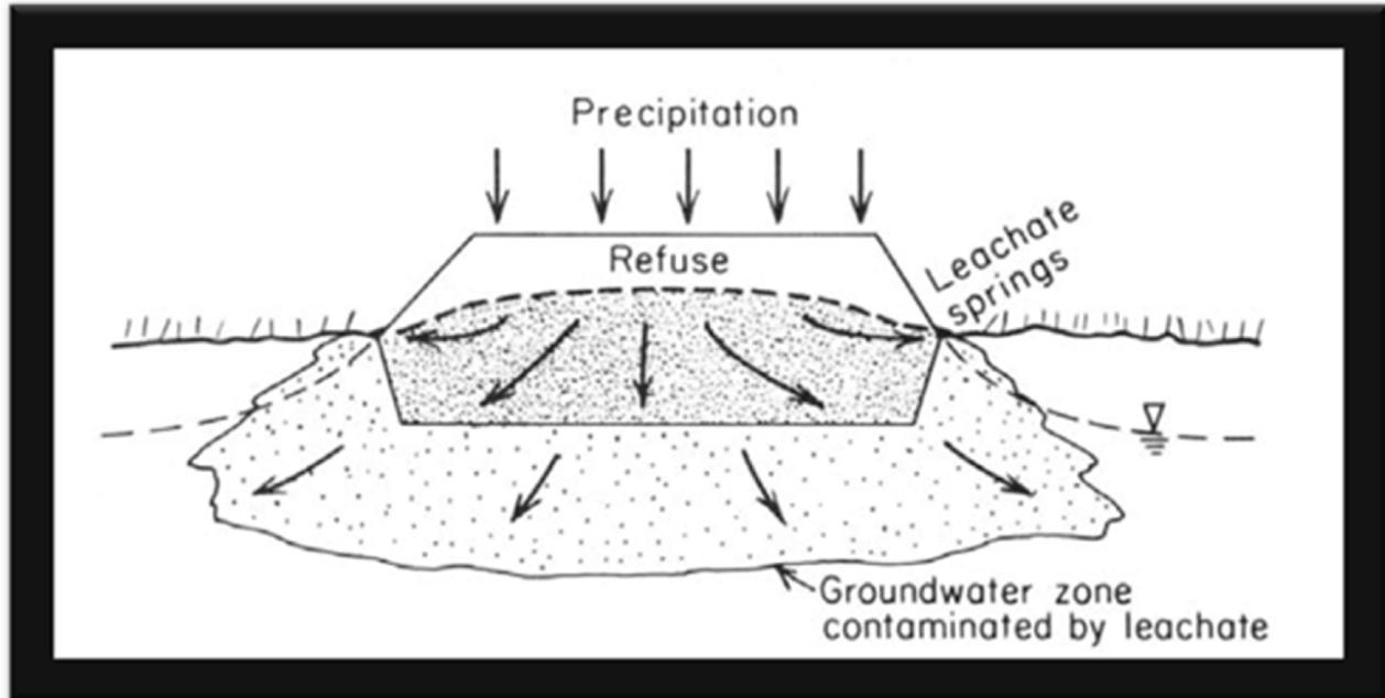
(Fig 1) Conceptual diagram of leachate migration from a typical landfill [9].
