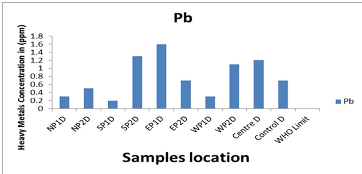
Fig 3.03 A plot of lead concentration against sample location during dry season.
