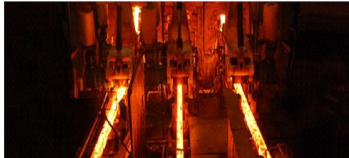
Billets are the best raw material to produce steel bars, as compared to ingots. Plant is capable of giving an output of 45 tons of billets in one heating. Given below is the production process.
