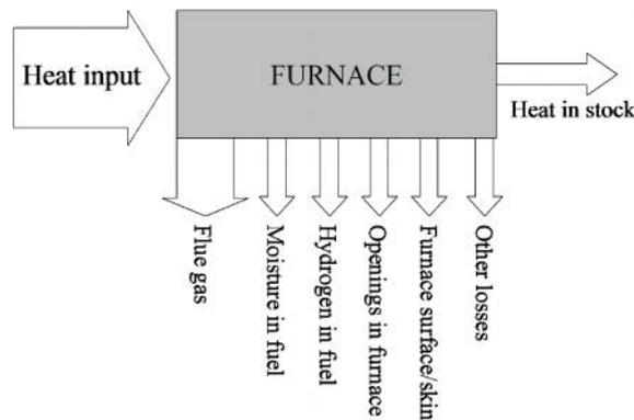
Ideally, all heat added to the furnaces should be used to heat the load or stock. In practice, however, a lot of heat is lost in several ways as shown in the figure.
