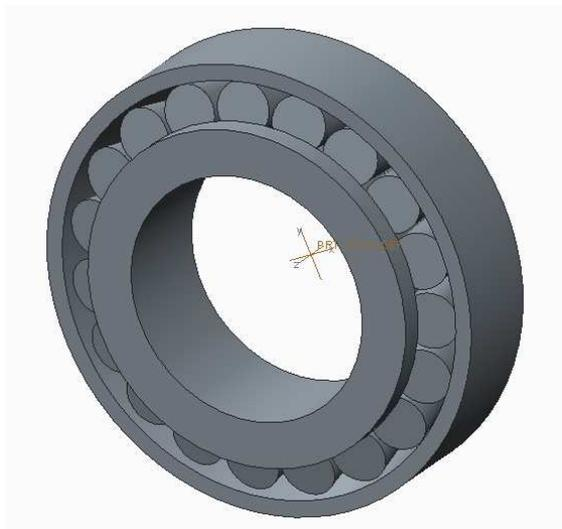
***Fig. 1. 3-D model of tapered roller bearing***
