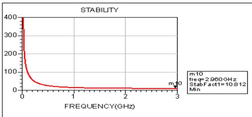
Fig. 7. Stability v/s frequency
