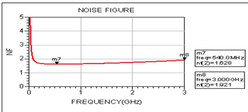
Fig. 5. Noise Figure over the operating frequency range
