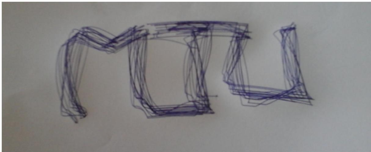
Fig. 17. Actual 2-DOF PM's Trajectory Planning of MTU
