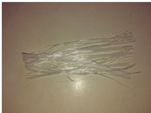
**Fig. 2. Commercial Nylon Fiber**
