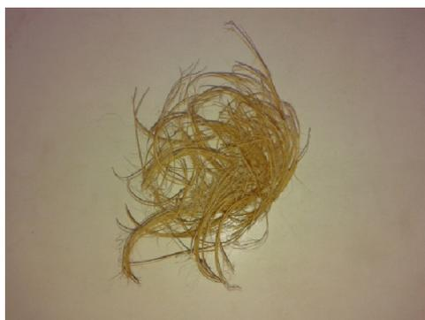
**Fig. 1. Extracted Areca Nut Fiber**
