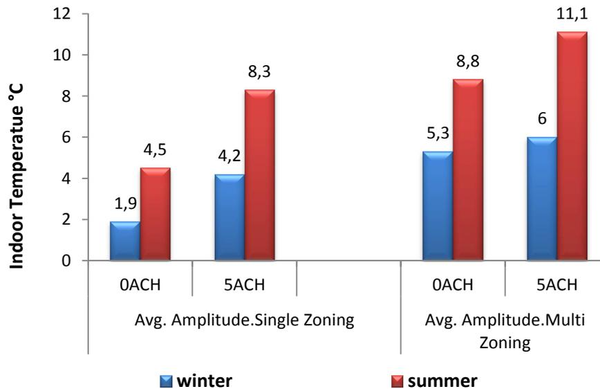
Fig. 9. Variation of internal temperatures for both configurations in winter and summer
