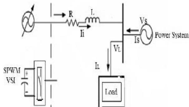
**Fig. 1. Standard Voltage Source Converter Scheme**
