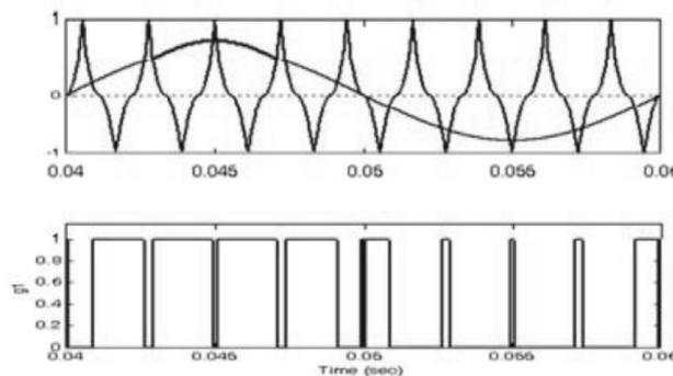
Fig. 3. Firing pulses generation in the proposed ISPWM Technique
