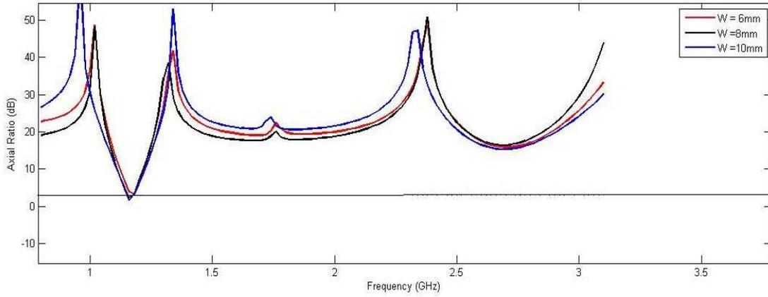
Fig.4. Simulated axial ratio for different stub width
