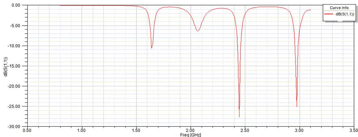
Fig.3. Simulated return loss for proposed antenna
