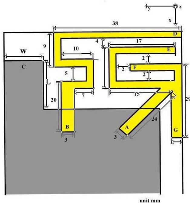
Fig.2. Detailed dimension of the proposed design
