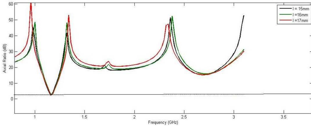
Fig.5. Simulated axial ratio for different stub length
