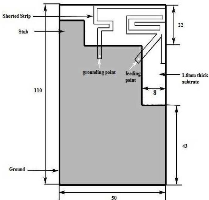
Fig.1. Geometry of the proposed design
