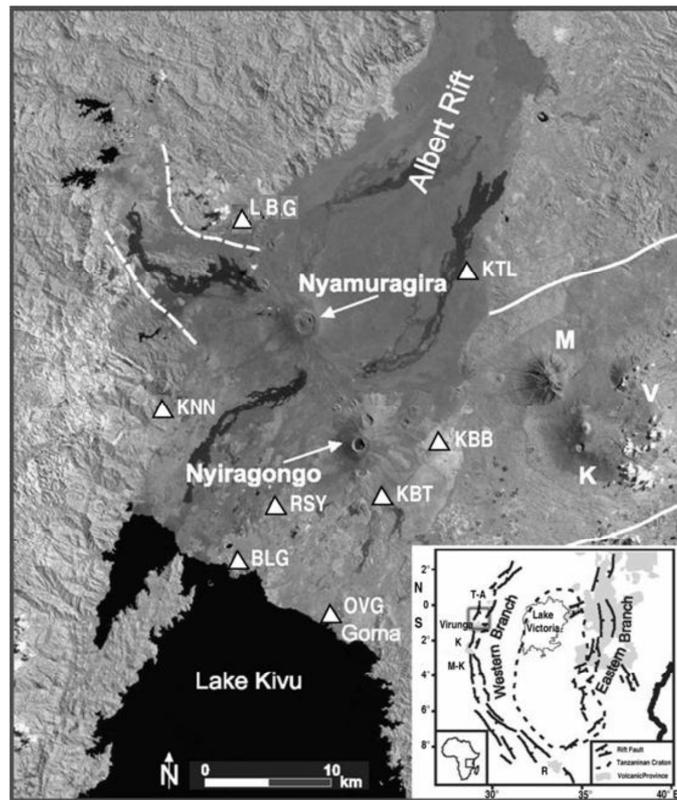
**Fig. 2.** Seismic network of the Goma Volcano Observatory. Seismic stations are marked by white triangles (Goma-OVG, Kunene-KNN, Rusayo-RSY, Bulengo-BLG, Kibumba-KBB, Kibati-KBT, Katale-KTL, Luboga-LBG).
