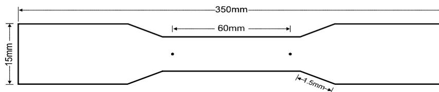
**Figure 1 Schematic diagram of tensile test sample**
