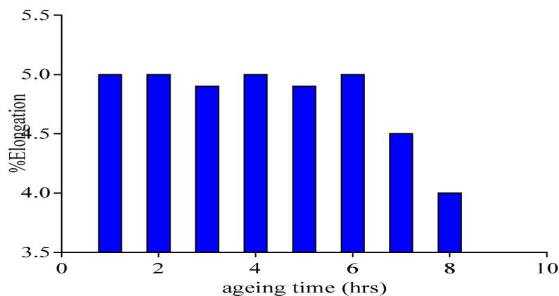
**Figure 4 Effects of ageing time on the ductility of samples 160 °C**
