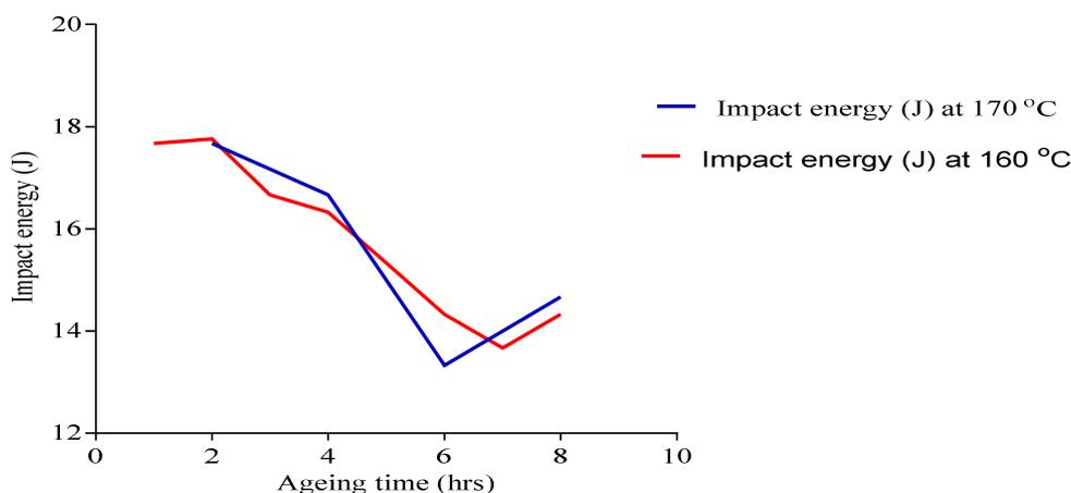
Figure 7 Composite curves of impact energies at 160°C and 170°C for Al-Si-Mg alloy
