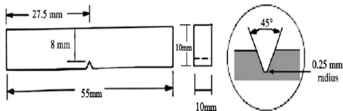
Figure 2 Schematic of impact test sample
