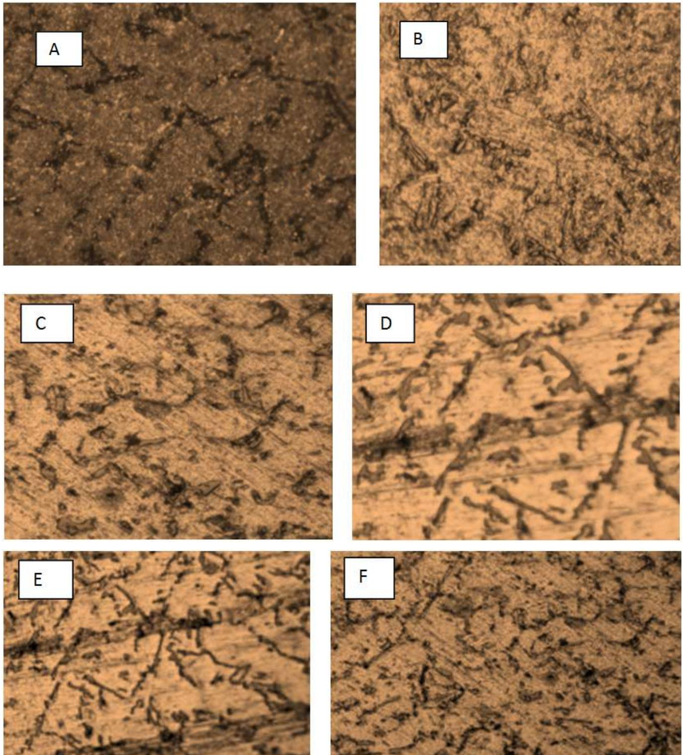
*Figure 10 Optical microstructures of Al-Si-Mg (a) as cast (b) SHT for 6 hours (c) aged 5 hours (d) aged 7 hours at 170 °C, (E) aged 6 hours and (F) aged 7 hours at 160 °C (x200).*
