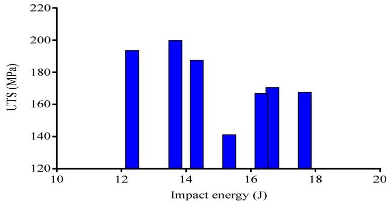
Figure 8 Bar charts of UTS against impact energies at ageing at 160 °C (Al-Si-Mg alloys)
