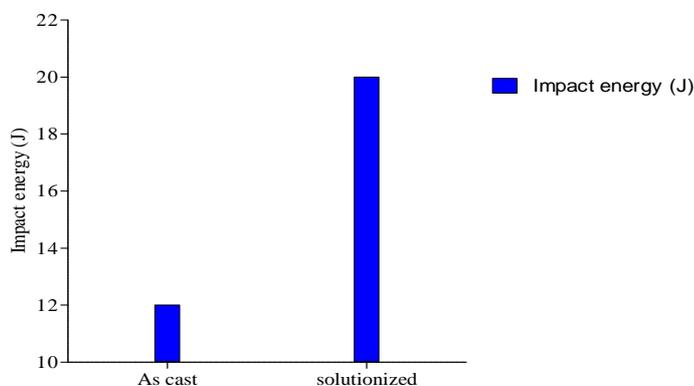
Figure 6 Impact energy of as-cast and solution treated sample
