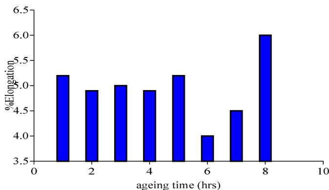
Figure 5 Effects of ageing time on the ductility of samples at 170°C
