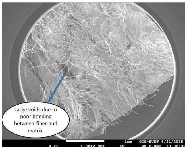
**Fig. 11. SEM Micrograph of Tensile Fracture Surface of 20% Fiber Reinforced PP Composite**
