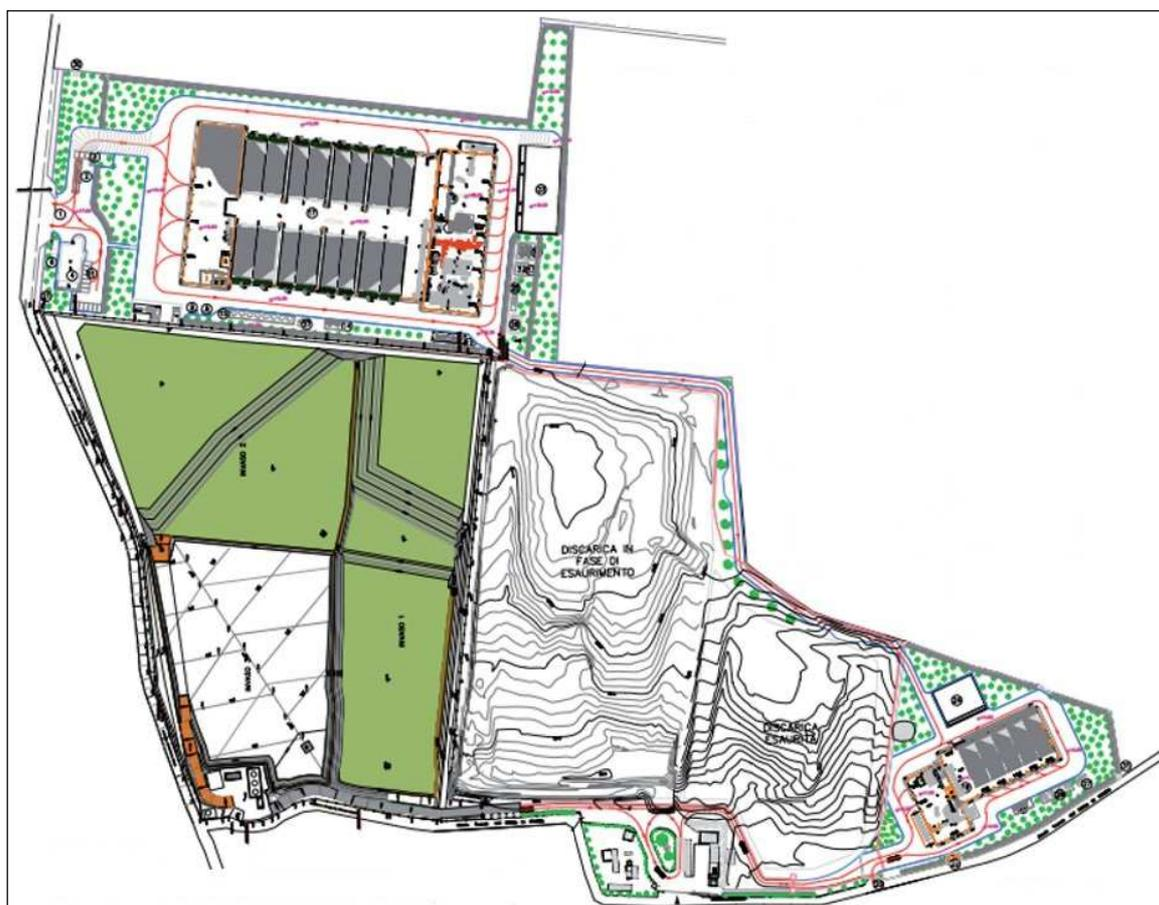
**Fig.11. Present situation of Andria MSW bio-mechanic-chemical treatment plant with Section B) landfill almost exhausted (bottom left)**
