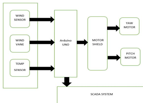
**Fig.1 Block Diagram Representation of the System**
