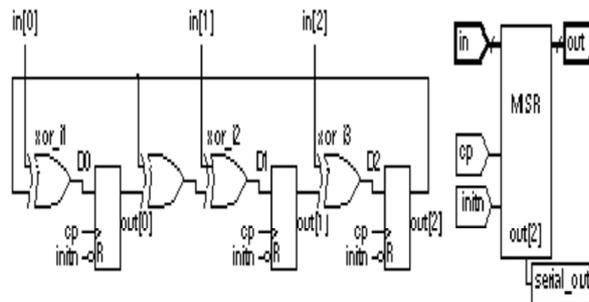
**Fig. 3 Multiple Input Signal Register**
