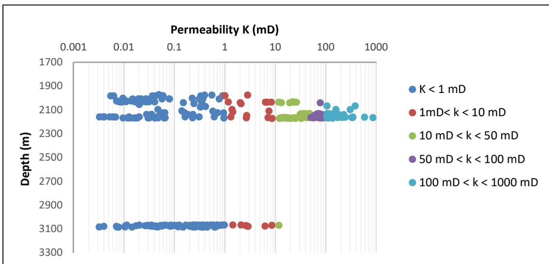
Fig. 2. Diagram of permeability variation versus depth in the FE-1 well
