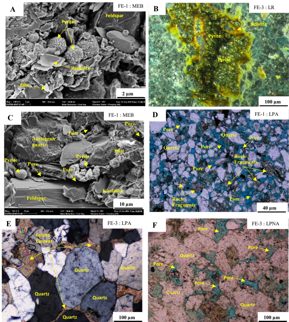
Fig. 11. Photomicrographs of authigenic minerals and pores from wells FE-1, FE-2, and FE-3. Presence of calcite (E), authigenic quartz (F), pyrite between the detrital minerals. Porosity blocked by calcareous cement (E), moderate (C, F) and good (D).
