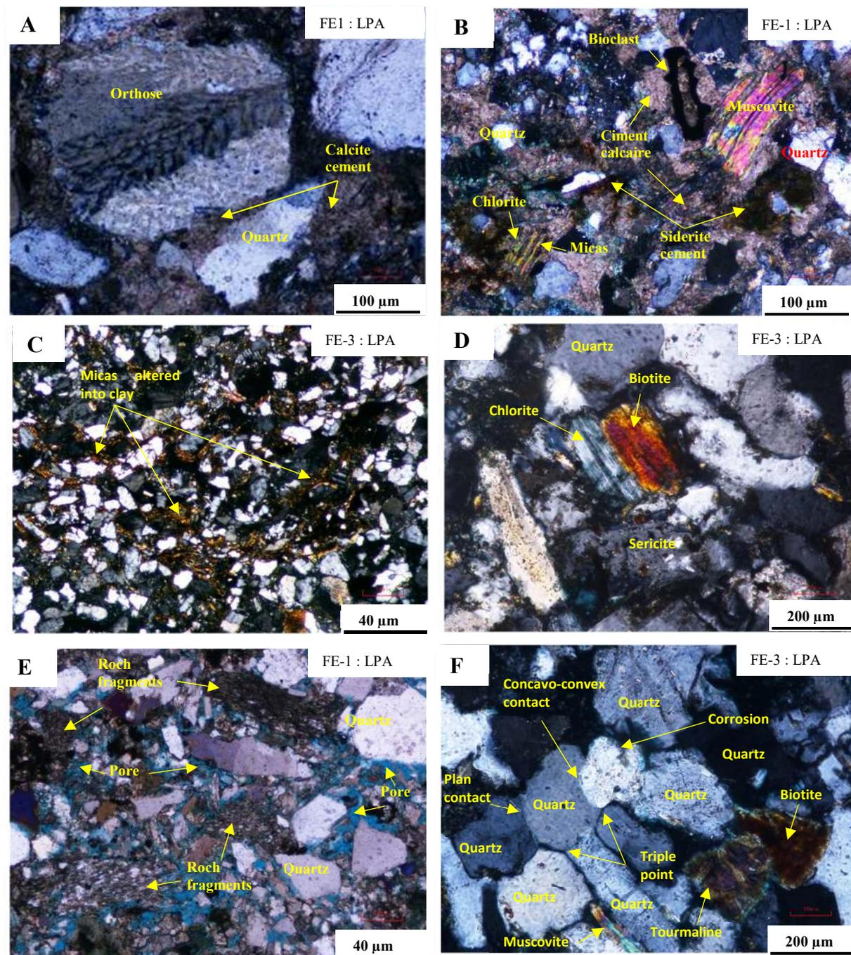
**Fig. 10.** Photomicrographs of detrital minerals from FE-1, FE-2, and FE-3 wells. Alteration of Orthosis marked by a single macle (A). Alteration of mica in chlorite (B, D) and clay (C). Flattened rock fragments (E), sandstones showing concavo-convex contact, plan contact and triple points (F). Tourmaline and biotite trapped between quartz grains (F).
