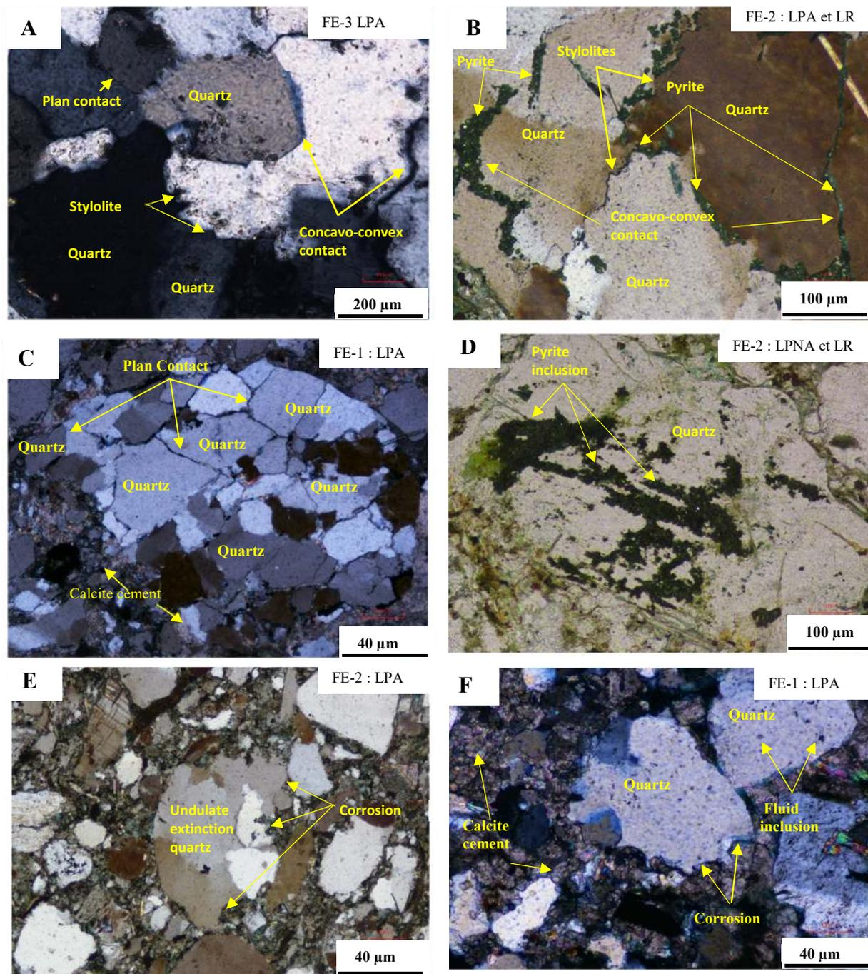
**Fig. 8.** Photomicrographs of sandstones of FE-1, FE-2, and FE-3 wells showing the enmeshed boundaries marked by the concavo-convex contacts and stylolite surfaces (A, B) and the straight boundaries shown by planar contacts (C). These limits contain iron oxides (pyrite). Corroded quartz grains with undulate extinction (E) and pyrite (D) and fluid (F) inclusions.
