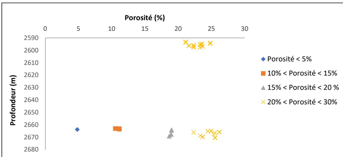
Fig. 6. Diagram of porosity variation versus depth in the FE-2 well
