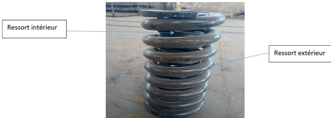
**Fig. 2.** *Ressorts de suspension des locomotives U 22C*
