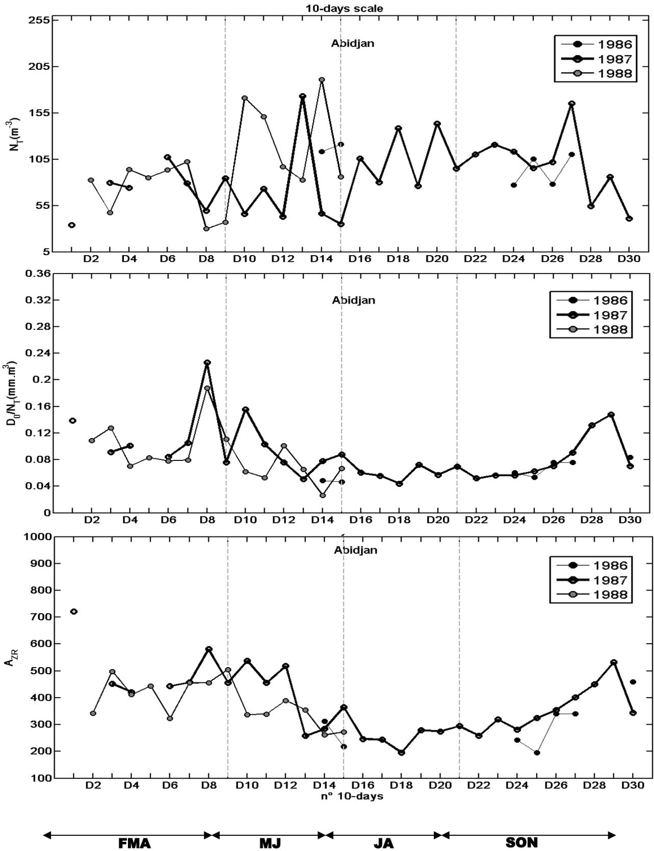
Fig. 4b. Idem Fig. 4a, but for the total number of drops  $N_T$ , the ratio between the diameter and the number of drops  $D_0/N_T$  and the pre-factor  $A$  of the power law Z-R
